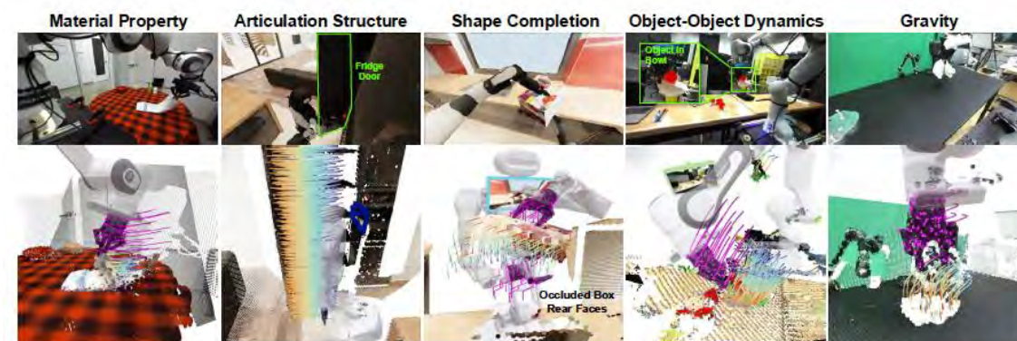
Figure 3. Rich Supervision of 3D World Modeling for Physical Interactions, when conditioned on 3D robot point flows and partial observable RGB-D. The 3D world modeling objective enjoys dense pixel-level supervision while encoding a wide range of capabilities central to robotic manipulation. To predict full-scene evolution, the model needs to implicitly segment objects of interest, identify material property and/or articulation structure, perform implicit shape completion for contact reasoning, propagate robot-object interaction for object-object dynamics, and simultaneously considering the effects of gravity, encapsulated all in a single forward pass of the learned model.
